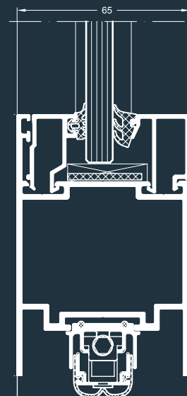
Schüco Tür ADS 65.NI FR 30, M = 1:2 Schüco Door ADS 65.NI FR 30, scale = 1:2
